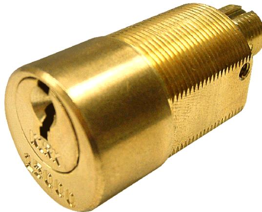
The Camlock is a compact, threaded cylinder interlock designed to fit smaller-sized switchgear. The key is trapped or released according to the position of the cam. It is designed to be installed with provisions or bracketry provided by the breaker manufacturer. The Camlock can be linked to other camlocks with the proper bracketry.
